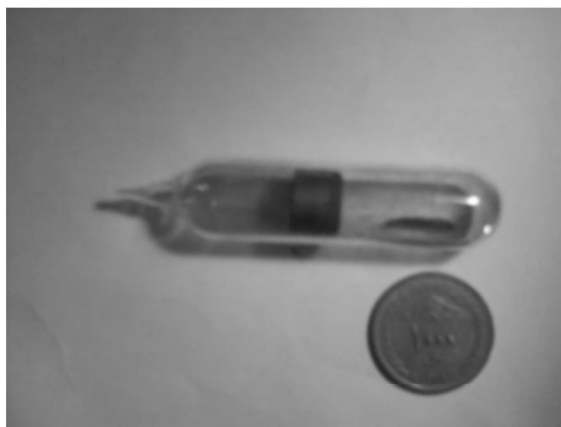
Fig. 1. Encapsulated sample by quartz before reaction in the furnace
